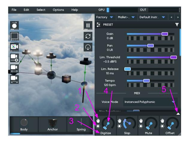
1. **Drag and Drop Handle** = Click and drag from this handle onto the 3D view to create an unconnected Macro object, or drag it onto a modulatable parameter in the Object Editor panel on the right side to connect it to that parameter on the selected objects (see the <u>Macro Drag and Drop</u> section below for a detailed explanation).
