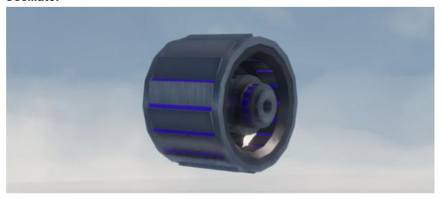
The oscillator is used to induce vibration based on a waveform in each of the body objects that it is connected to via an exciter link. The orientation of the oscillator controls the direction in which each body is vibrated.
