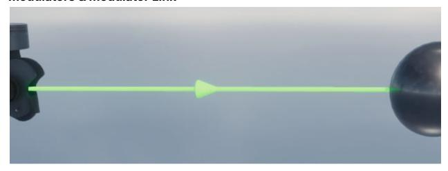
Every modulator uses a modulator link to connect to other objects. This link appears as a green line with an arrow indicating the direction data is being sent.
