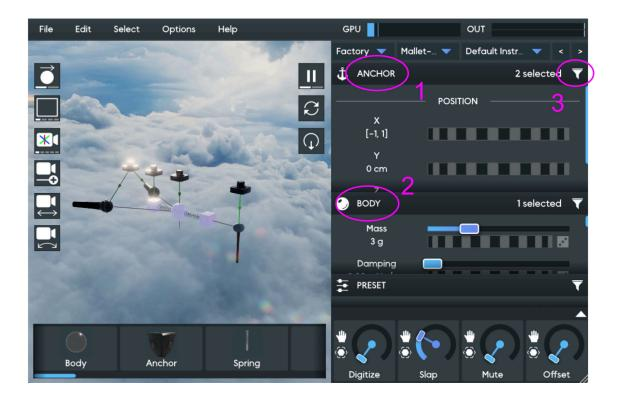
The object editor panels can be resized by dragging their headers up and down with the mouse. Double-clicking a header will maximize its size. Finally, clicking the Filter button labeled (3) in the diagram will filter the selection to only the given type of object.
