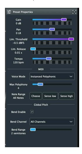
**Gain** = The amount of gain that will be applied to the master output signal
