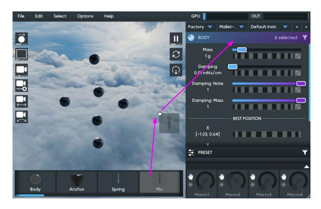
☑ **TIP:** For some kinds of objects, using the "C" hotkey to connect them will result in a different type of link depending on which direction you make the connection. For example, connecting from an Envelope Follower to a Mic will result in a Modulator Link.
