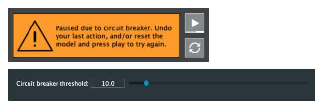
The circuit breaker is a type of failsafe mechanism that is built into Anukari to prevent a "flood" of volume from escaping the app (and into the user's speakers and/or ears.) It will automatically pause playback of Anukari's simulation engine whenever RMS loudness exceeds the level set by the Circuit Breaker Threshold setting in Global Preferences. Lower values make it more sensitive and therefore will trigger the failsafe more often. The recommended level is 10.0.
