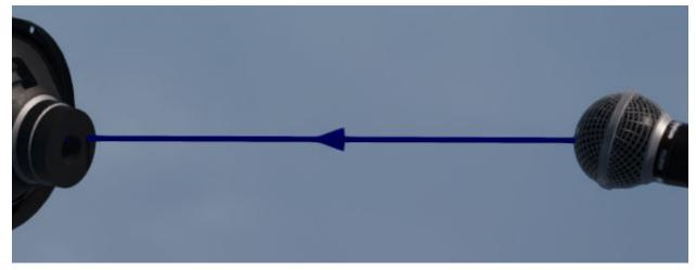
The delay line connects an audio input exciter or envelope follower to each of the mics from which it will receive an audio signal. They appear as blue lines with an arrow indicating the direction of audio signal flow. An audio input or envelope follower can be connected to many mics, and will sum the audio signal from all of them. The delay line link is used to configure the delay for each mic's audio signal.
