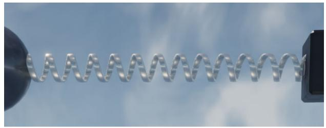
The spring physically connects body objects to one another and to anchors. Each spring has a configurable neutral length that it is always trying to return to. If it is stretched beyond its neutral length, it will pull the attached body objects together, and if it is compressed below its neutral length, it will push these objects apart.
