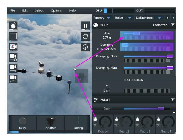
✓ **TIP:** The drag and drop system also works when dragging other kinds of modulators from the Object Palette. For example, you can drag an LFO from the Object Palette onto the Mass parameter in the same way that you can drag a Macro from its grab handle.
